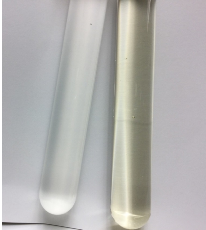
Figure 2: Bio-renewable polyester acrylate (left) versus petroleum polyester acrylate (right)
